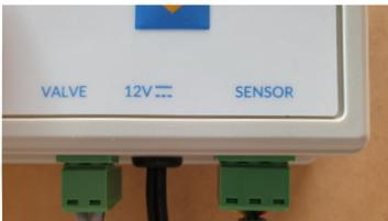
**NOTE:** Sensor and Solenoid plugs must face backwards when inserted into the new Water Witch Control Box.
