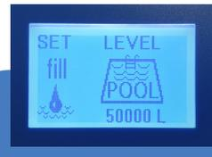
If you do not press **ENTER** to confirm the sensor level the unit will remain in **SET LEVEL MODE**.
